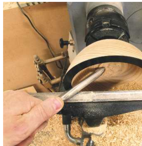
▲ Pic.13 A problem with the 45° angle on the tool is that it will become very difficult to keep the bevel in contact with the bottom of the bowl as you go deeper; the rim will get in the way. This is a job for the 60° tool, as you'll see later
